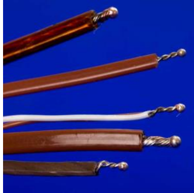
Pre-cut Validation Thermocouples
